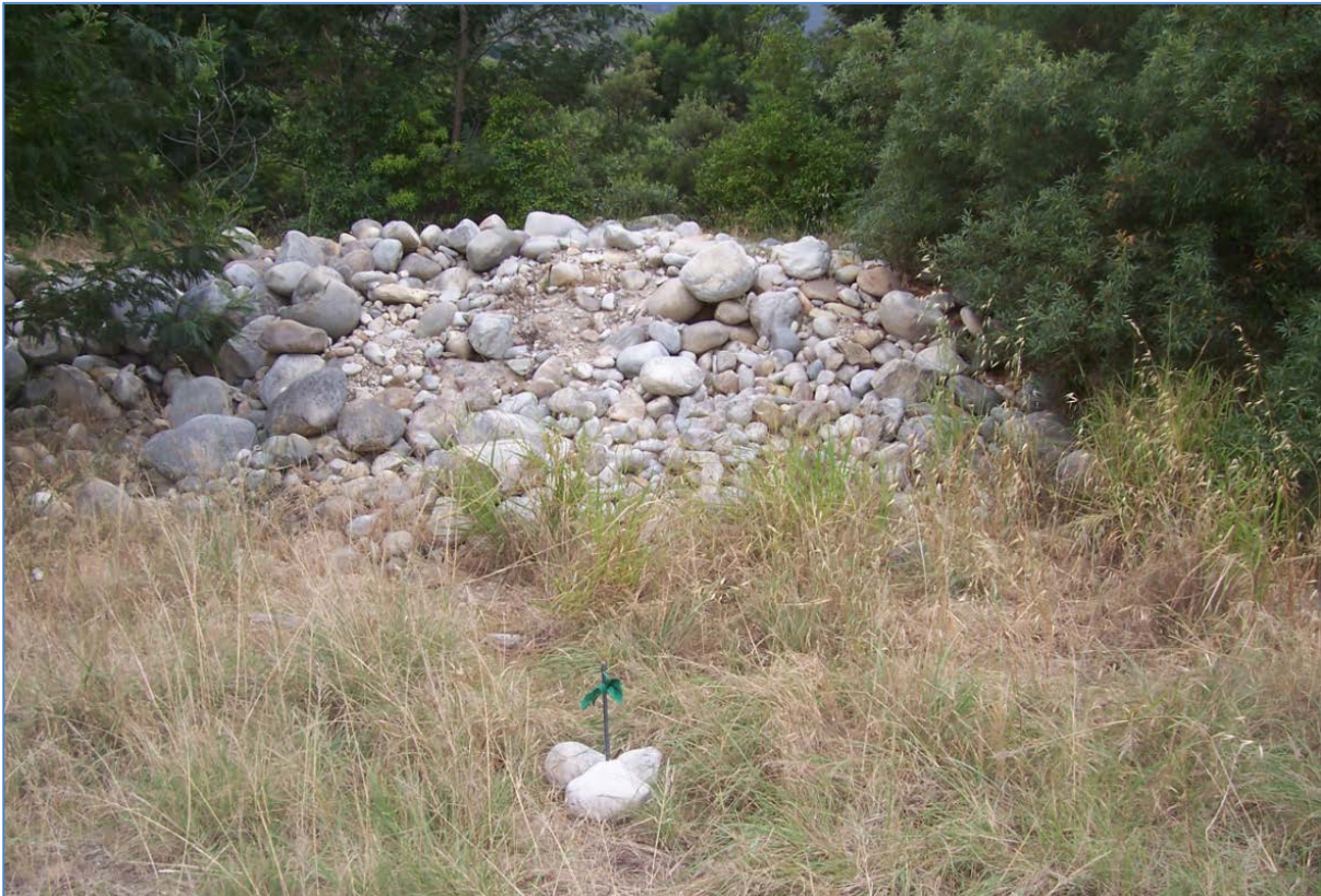
Figure 12: Typical Alluvial Sediments Excavated to Depths in Excess of 3m at Proposed Weir
